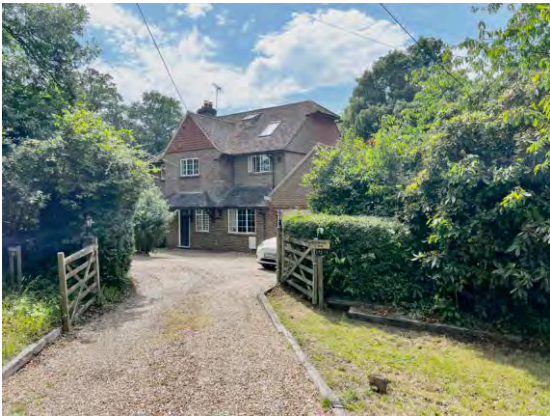
Half-hip (or Jerkinhead) roof form
