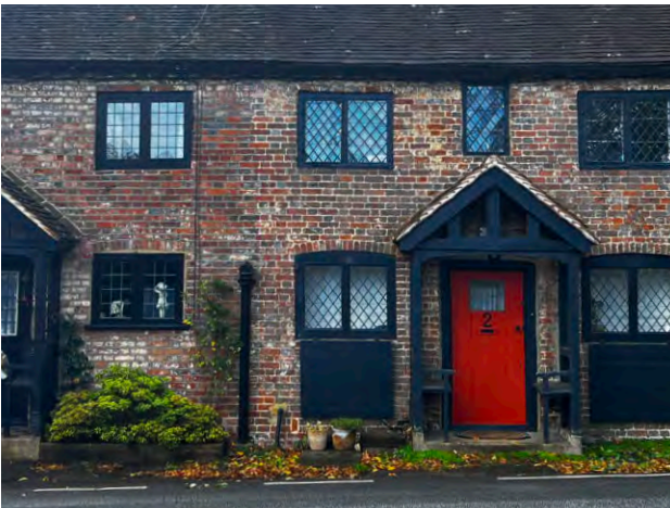
Brickwork - Often multi-bricks with a broad variation of deep red, russett and brown and guilt tones. Decorative courses include soldier and string courses, quoin banding and dental courses
