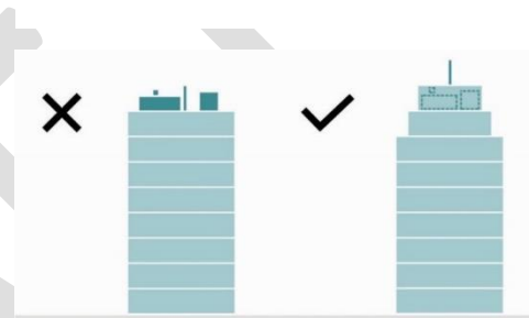
Figure 6: Use of appropriate screening to integrate rooftop building servicing features reduces visual prominence and harm to views.
