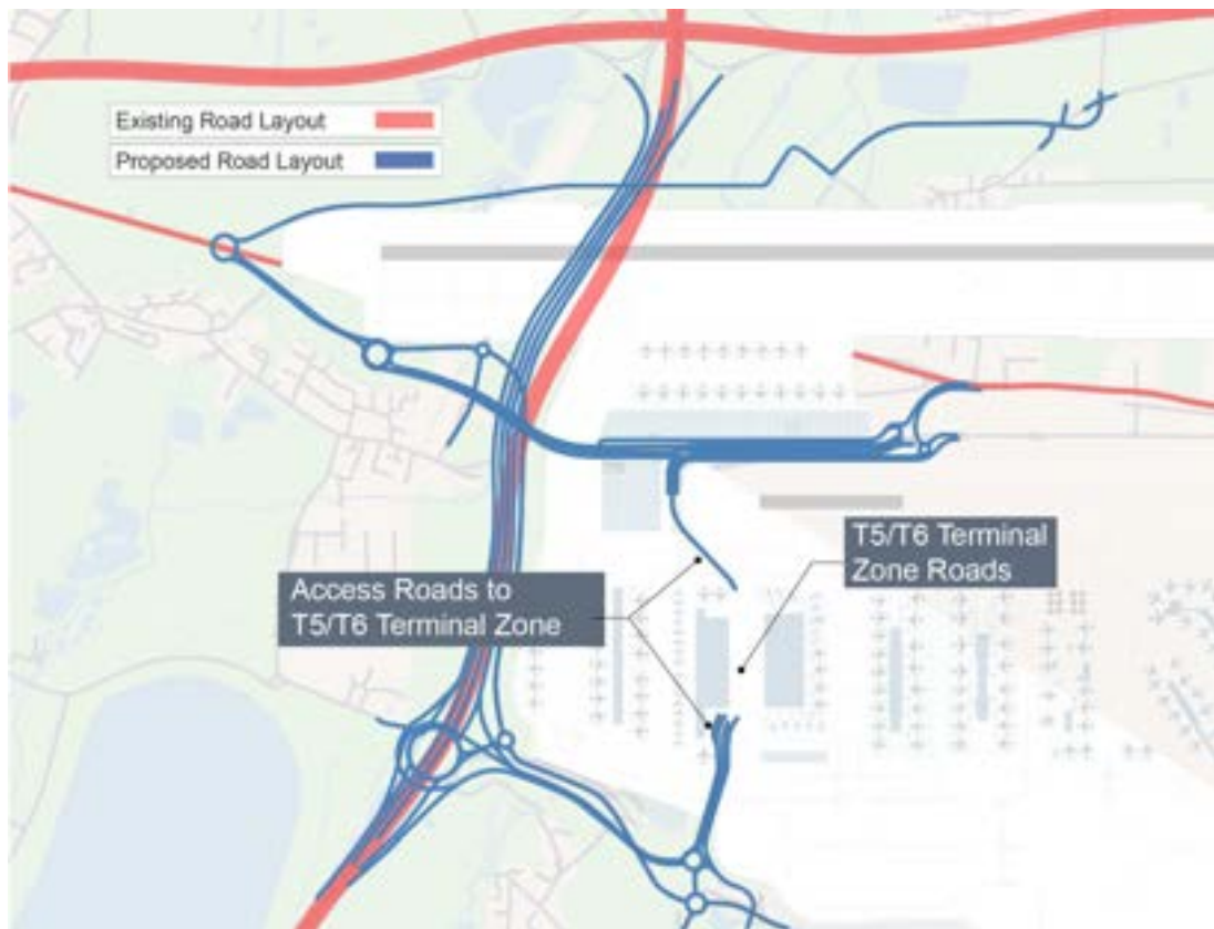
Figure 16. T5/T6 Terminal Zone Roads
