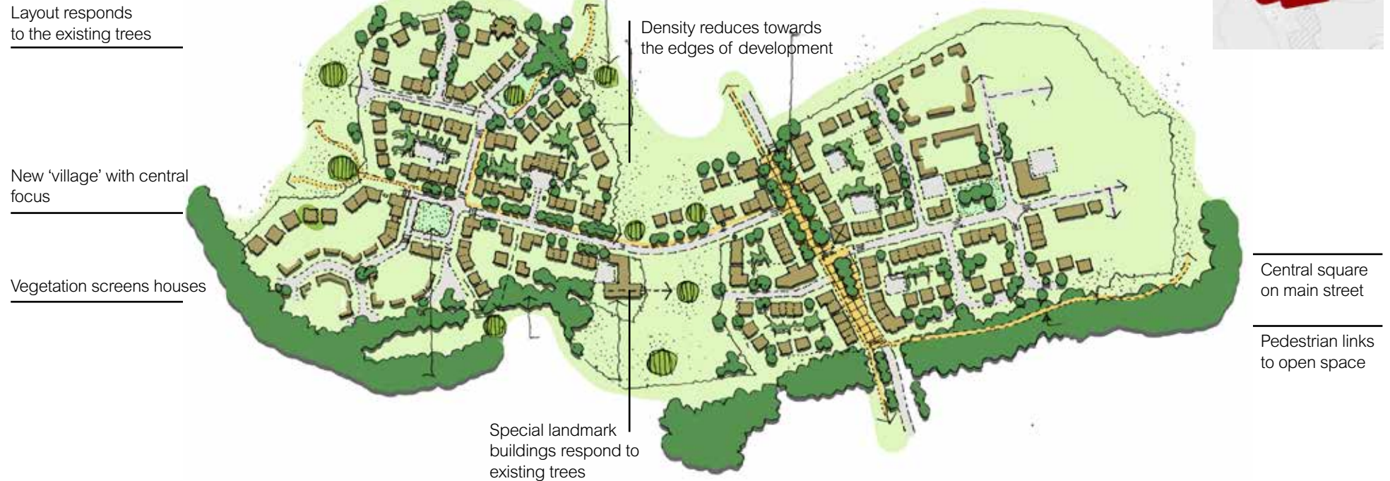
Fig 44: Illustrative drawing showing residential development in the south of the site. More intense built forms line the primary street becoming increasingly loose and more green towards the edges
