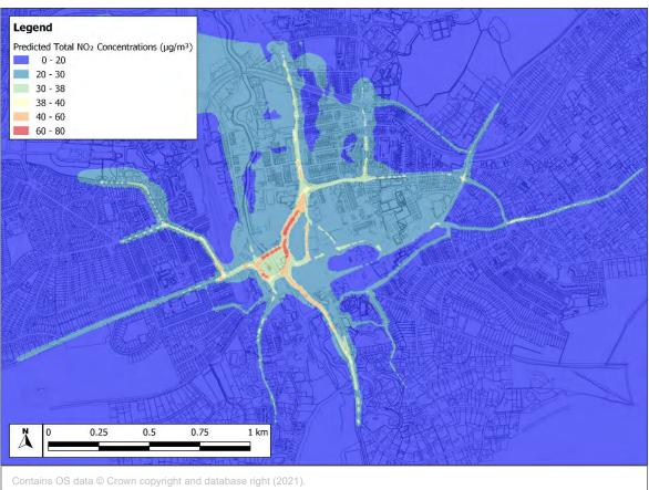
Figure 12: Contour Plot of Predicted NO<sub>2</sub> Concentrations
